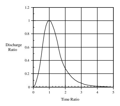
Figure 11.3: SCS Dimensionless Unit Hydrograph
