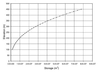
Figure 11.5: Storage vs. Elevation Relationship
