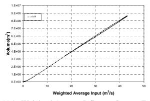
Figure 11.9c Weighted Average Influx *vs.* Storage Function - x = 0.09.
