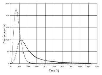
Figure 11.8: Level Pool Routing: Inflow and Outflow Hydrographs
