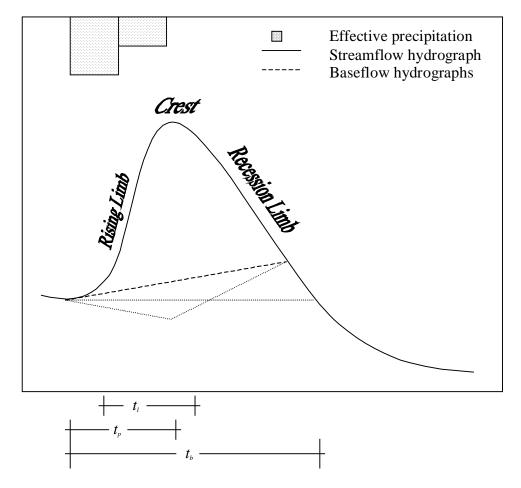
Figure 11.1: Schematic Description of Hydrograph
