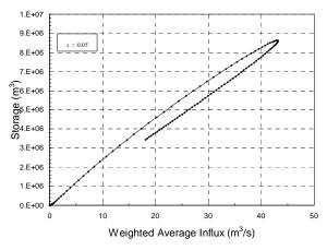
Figure 11.9a: Weighted Average Influx *vs.* Storage Function - x = 0.05.
