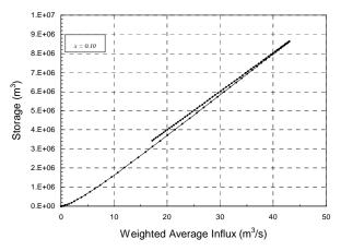
Figure 11.9d Weighted Average Influx vs. Storage Function - x = 0.10
