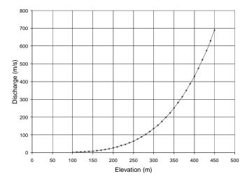
Figure 11.6: Elevation vs. Discharge Relationship
