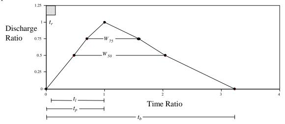
Figure 11.2: Snyder's Synthetic Unit Hydrograph
