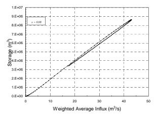
Figure 11.9b: Weighted Average Influx vs. Storage Function - x = 0.08.
